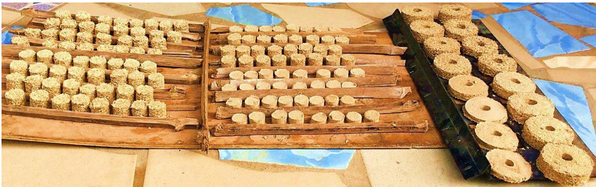
Figure 3: The samples of fuel briquettes produced from a blend of corncob and rice husk
