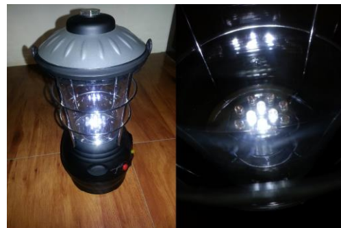
Figure 10: The first section of the LED settings, light up inside 4 LEDs
