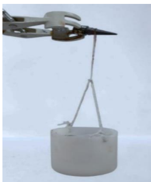
Figure 5 Apparatus assembly for Breaking load point
