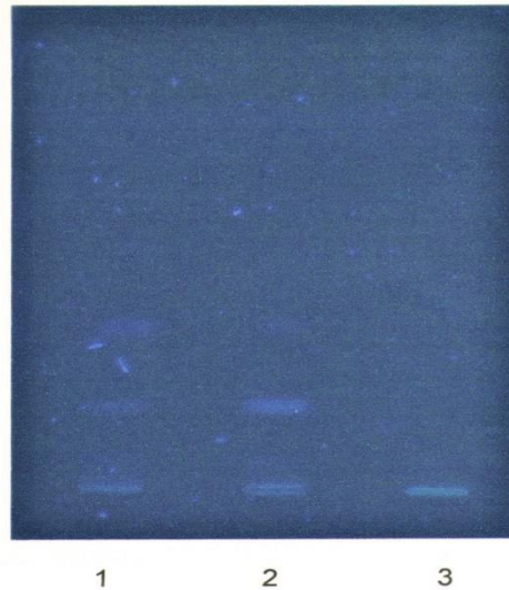
Fig.-3: TLC profile of whole plant extract of Convolvulus pluricaulis (1), Evolvulus alsinoides (2), and Clitoria ternatea (3).
