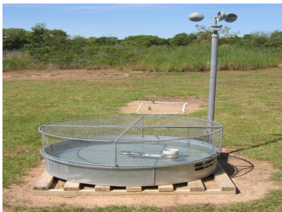
Figure 9: Class A evaporation pan with weather station and protective cage [24].
