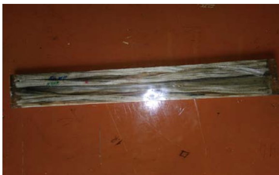
Fig: 2 shows the composite beam of Hemp and glass fiber composition.
