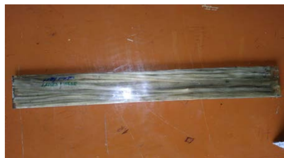
Fig: 1 shows the composite beam of ladies finger and glass fiber composition.
