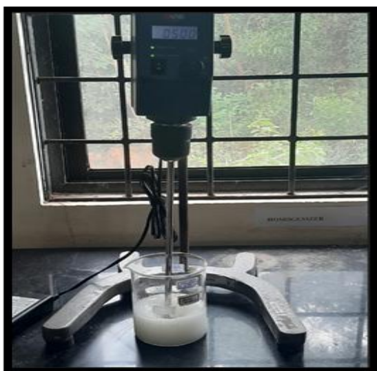
Fig 1: Preparation of microsponges by quasi emulsion solvent diffusion method
