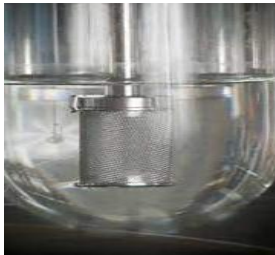
Fig 3: In-vitro drug release study using USP Type I Apparatus
