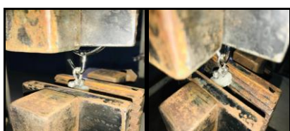
Figure: Specimen Clamped in The Universal Testing Machine
