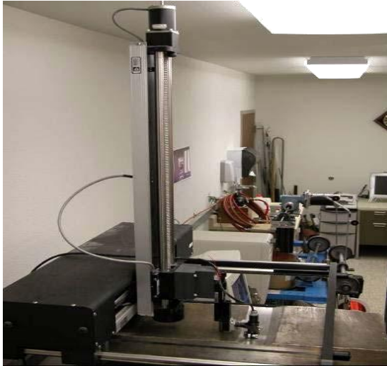
Fig 7. Eddy current testing setup
