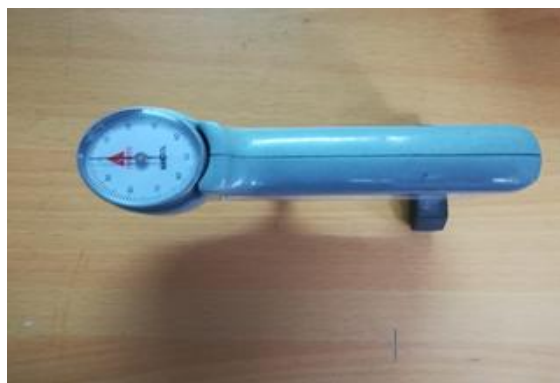
Fig 7: Barcol Hardness Tester
