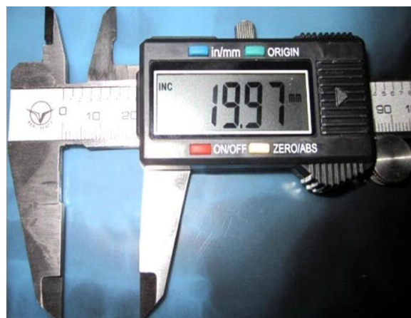
Figure 1: Measurement of interpedicular distance from digital Vernier caliper.
