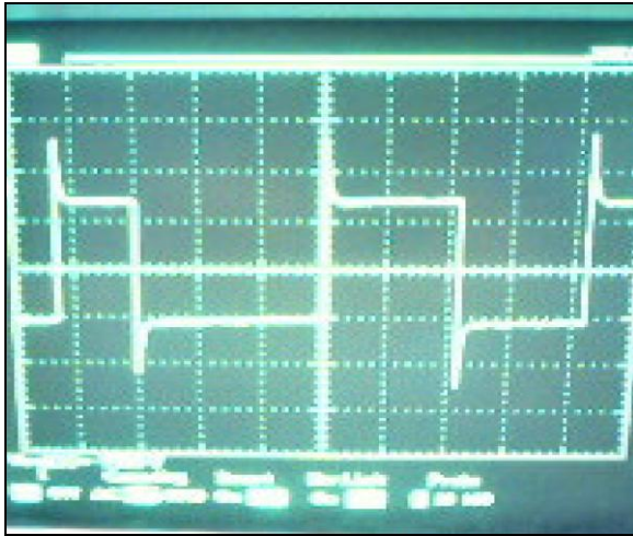
Figure 11: The output waveform of fixed direction transistor Q2
