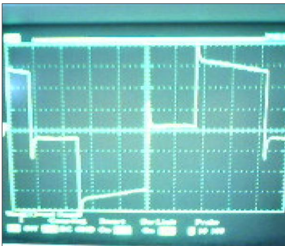
Figure 8: Inverter output voltage waveform
