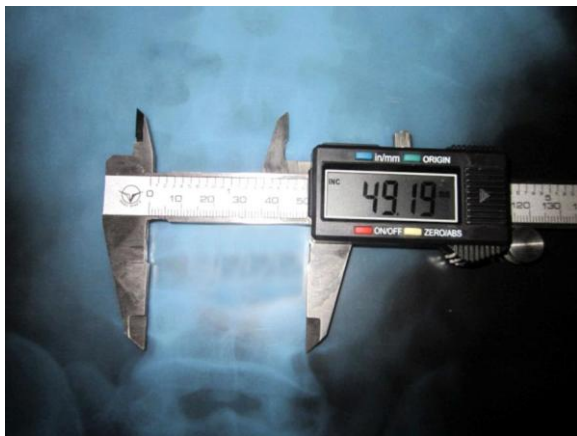
Figure 3: Showing measurement of transverse diameter of lumbar vertebral body by digital vernier caliper.
