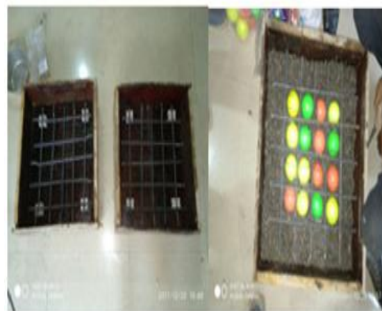
Figure 1: Cover and specimen Reinforcement
