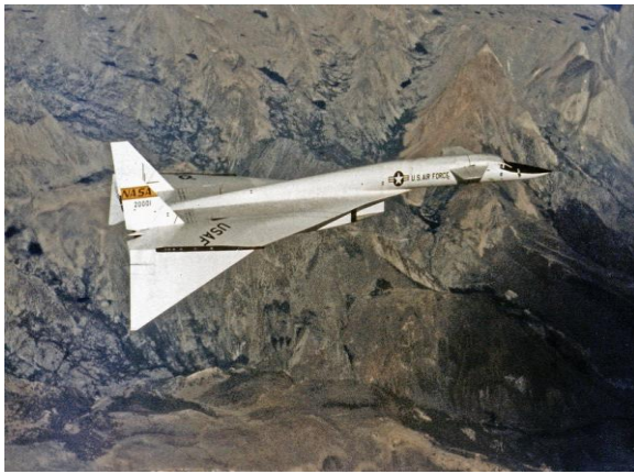
Fig:2A-XB-VALKYIRE(first plane to adopt span adaptive wing concept)
