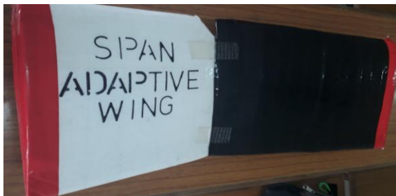
Fig:3M-Wing which was tested in wind tunnel (scaled down).
