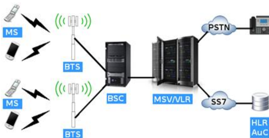
Figure 1 : Basic Structure and Component of Mobile Network
