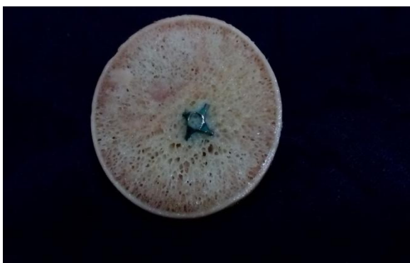
Fig 3: Cut section of cadaveric femoral head after insertion of Helical blade.
