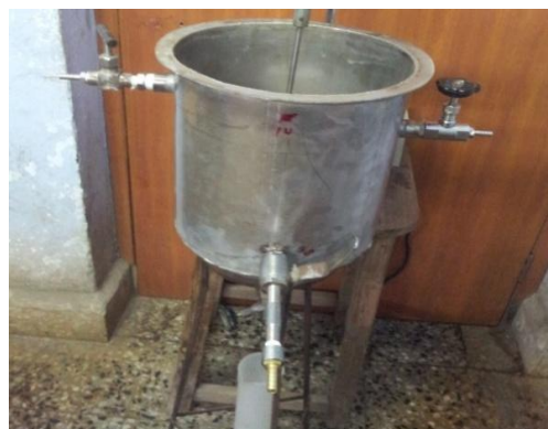
Fig 1: Activated Sludge Tank
