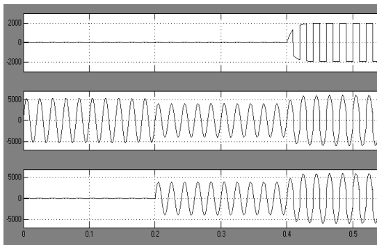
Fig.5 Voltage across external, LOAD-1 &LOAD-2 waveforms
