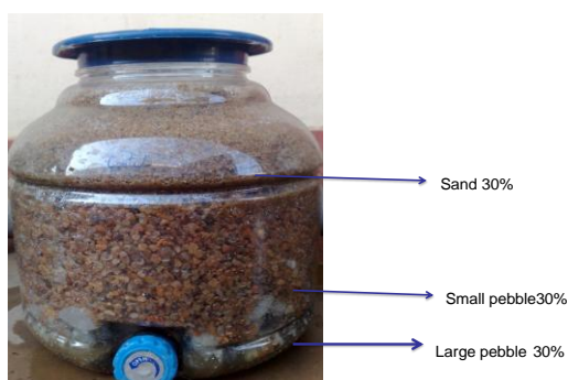
Figure 7. Filter system (Control) to check the Phytoremediation properties.
