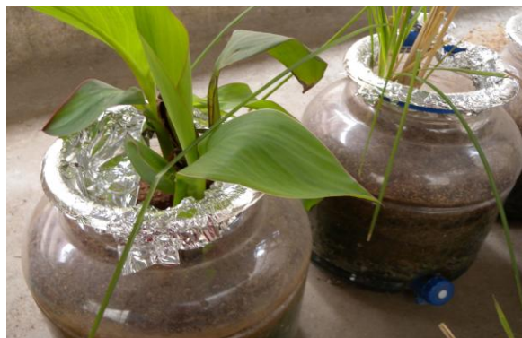
Figure 6. Filter system to check the Phytoremediation properties of Canna indica .
