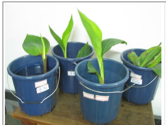
Figure 8. Simulated Hydroponic technique for phytoaccumulation study.
