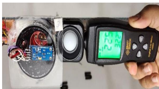
Figure 5. Testing the GY-30 Lux Sensor Reading Results against the Lux Meter 5.1.2. Sensor_Lux Reading Percent Error Testing
