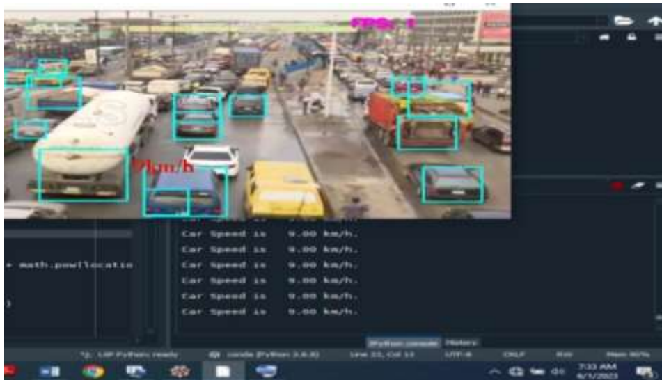
Fig. 12: Speed estimation as Heavy traffic (0-14km/hr) (Output from Python Program)
