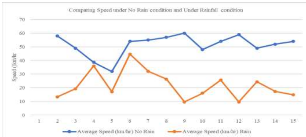
Fig.3; Vehicle Speed during dry weather is higher compared to wet weather for June, 2018.
