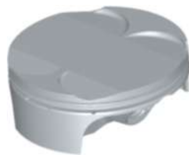
Figure 1. Piston for KTM 450 motorbike engine.
