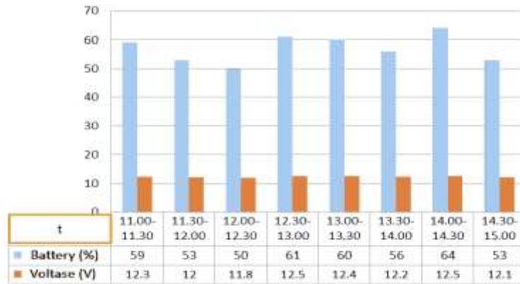
Figure 8. Battery Percentage and Battery Voltage Diagram on DC Lamps
