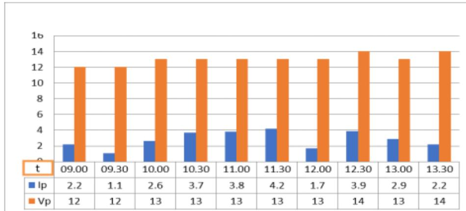
Figure 2. Current and Voltage Data Diagram on Solar Panels Against Time
