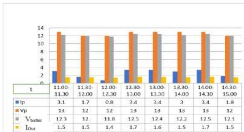
Figure 7. Diagram of incoming current, outgoing current, input voltage, and output voltage on a DC lamp
