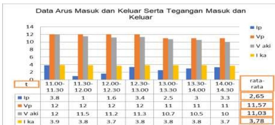
Figure 5. Incoming and Outgoing Current Data Diagram and Incoming and Outgoing Voltages on AC Lamps
