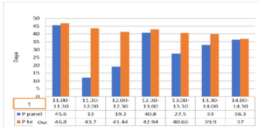
Figure 6. Incoming Power and Outgoing Power Diagram for an AC Lamp
