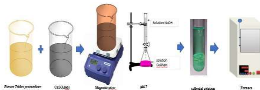
Figure 2. Flowchart of CuONPs synthesis via green synthesis method
