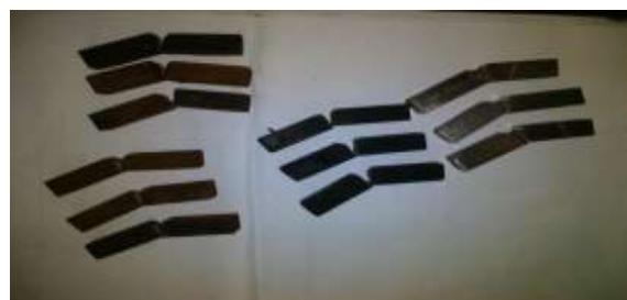
Figure 9. Impact test material after testing process
