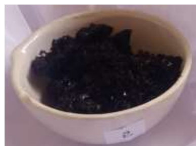
Figure 7. Powder sample after heating in a muffle furnace.
