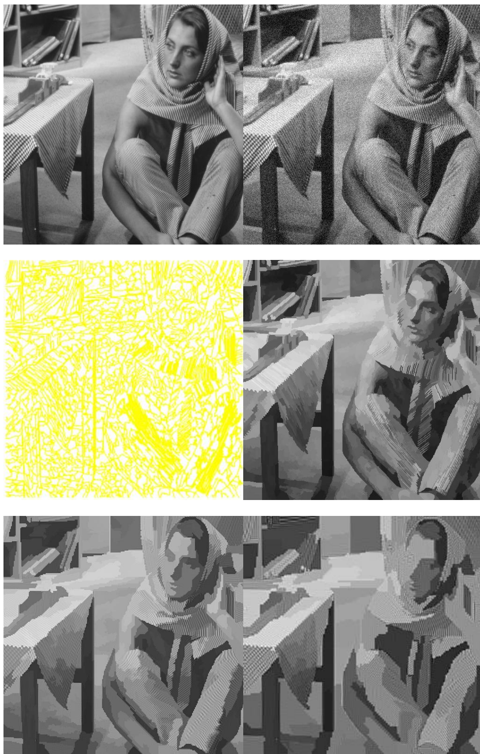
A)original image, B)noisy image, C)segmented image, D)region merging level 0 , level 1 , level 2 .
