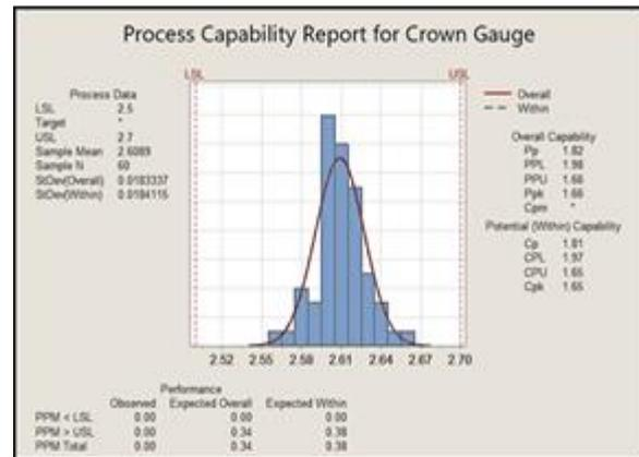
**Fig. 3. Process Capability for Crown Gauge Dimension**
