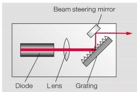
Fig.1: Schematic view of ECDL scheme
