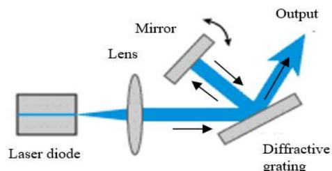
Fig.3: Schematic view of Littman configuration of ECDL system
