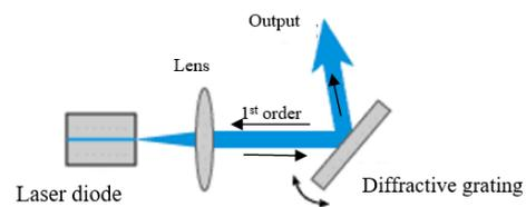
Fig. 2: A schematic view of Littrow configuration the ECDL system
