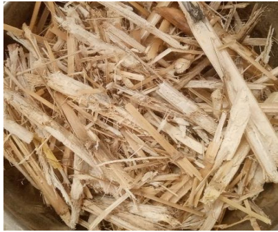
Figure 3: Poorly graded fibers
